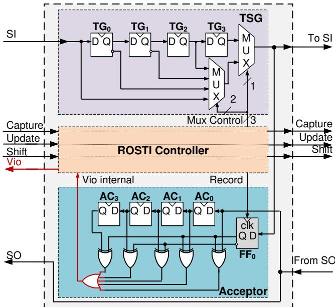
Fig. 5. Detailed architecture of ROSTI
