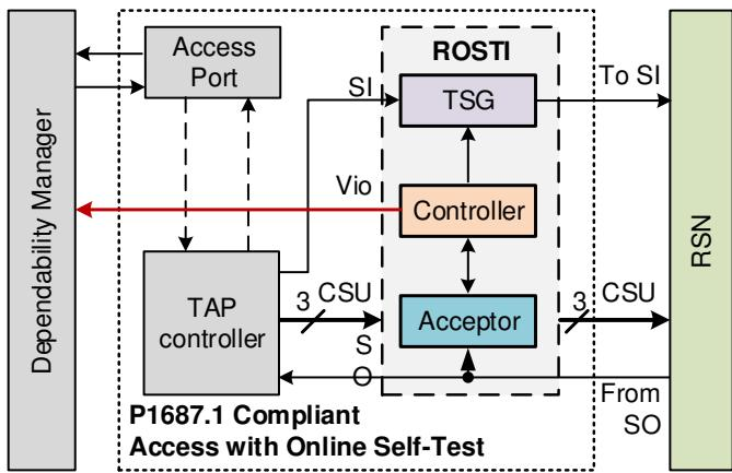
Fig. 3. The ROSTI scheme for online RSN test
