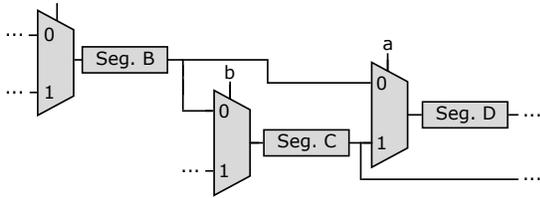
Fig. 5. Vicinity of scan segment B from fig. 2 after the first two steps of the final synthesis. The multiplexer address signals, such as a and b, are yet to be connected.
