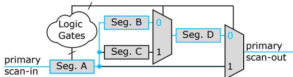
Fig. 2. A reconfigurable scan network with scan segments A, B, C, D. Segments A, B, D are on the active path (light blue) in the initial state.
