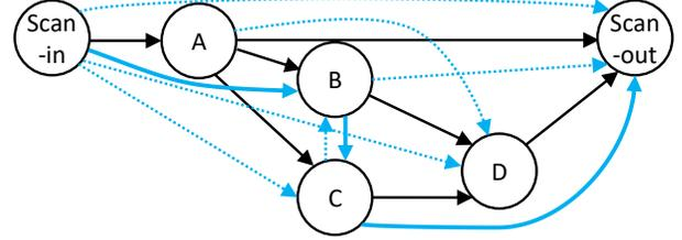
Fig. 4. Potential edges (dotted and solid) and vertices of the RSN in fig. 2. Edges of the dataflow graph are colored black. The edges of the minimal augmenting edge set  $E_A$  computed by the ILP have solid lines (black and light blue).
