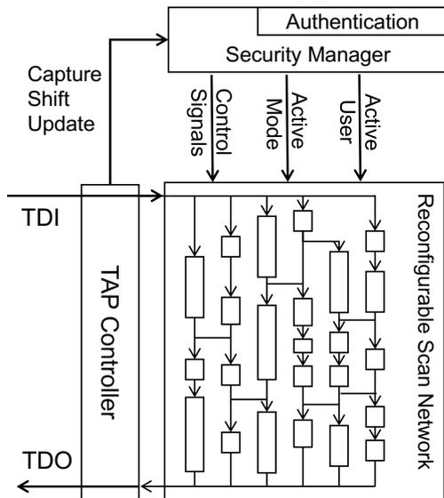
Figure 1. Overview of the architecture consisting of the test access port (TAP), the security manager, and the reconfigurable scan network.
