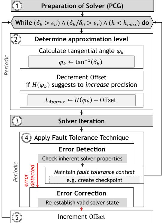
Figure 2. Overview of our technique for the Preconditioned Conjugate Gradient Solver (PCG).
