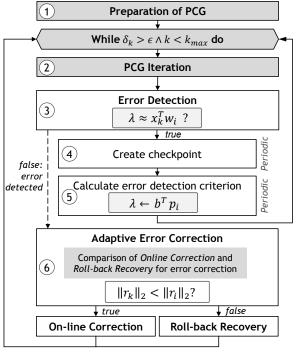
Figure 1. Overview of the Fault-Tolerant Preconditioned Conjugate Gradient Algorithm.
