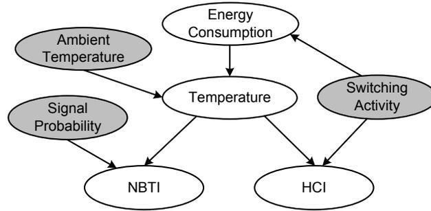
Fig. 6. Relation between NFP models for aging prediction (shown in white) and the required observables (shown in grey)
