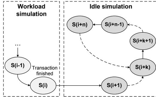
Fig. 2. Loop fast-forwarding for idle cycles
