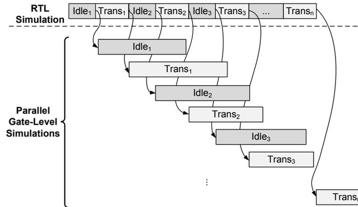
Fig. 3. Parallel gate-level simulation example. The stimuli and initial logic states are generated by RTL simulation.
