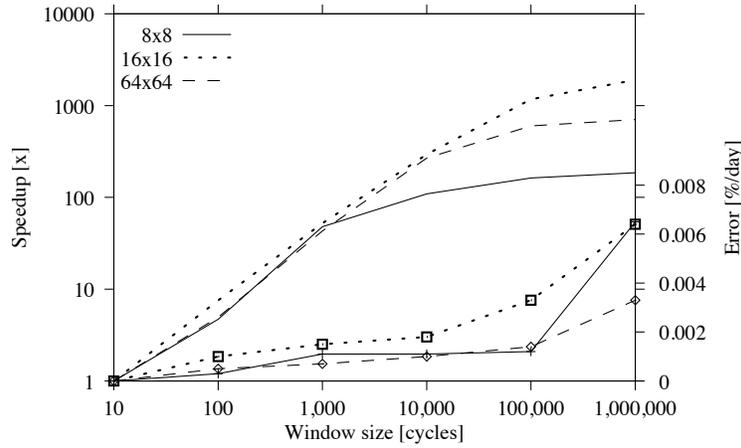
Fig. 10. Overall speedup vs. window size for IDCT core
