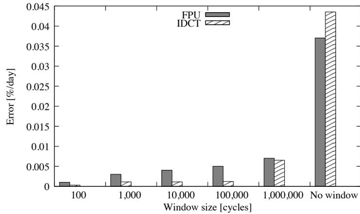
Fig. 11. Relative error with random input patterns for NBTI degradation
