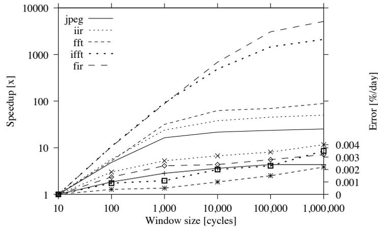
Fig. 9. Overall speedup vs. window size for FPU core
