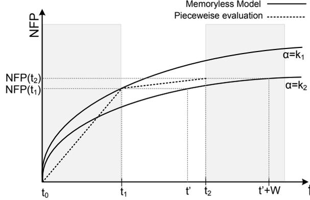
Fig. 5. Piecewise NFP evaluation example
