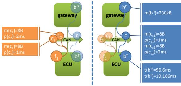
**Figure 6: The message  $c$  is only active, if the functional task  $t_1$  as well as its messages  $c_1$  and  $c_2$  are inactive. By mirroring their sending patterns, the test patterns can be transmitted transparently for other subscribers.**
