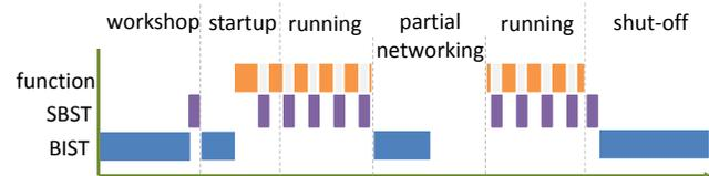
**Figure 1: The applicability of advanced diagnostic features depends on the operational mode of the automotive system.**
