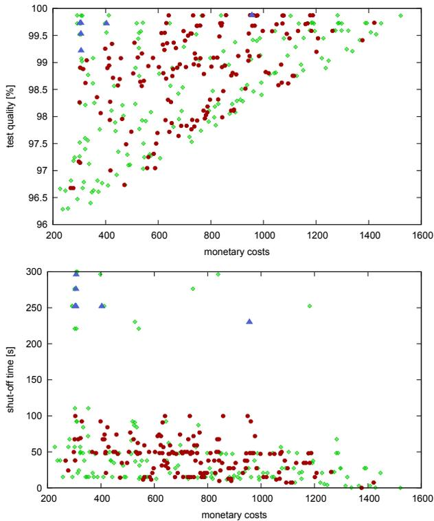
**Figure 7:** 322 implementations showing the tradeoffs between monetary costs  $\Phi$  versus test quality  $Q$  (top) and monetary costs  $\Phi$  versus shut-off time  $O$  (bottom). Implementations with three of four applications with fulfilled safety goal are marked with  $\diamond$ , remaining implementations with shut-off time less than 200 seconds are marked with  $\bullet$ , implementations with higher shut-off time are marked with  $\blacktriangle$ .
