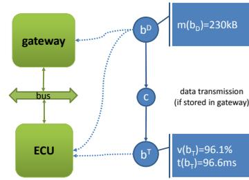
Figure 4: The BIST data task  $b^D$  can be mapped to the gateway or to the same resource as the corresponding BIST test task  $b^T$ .
