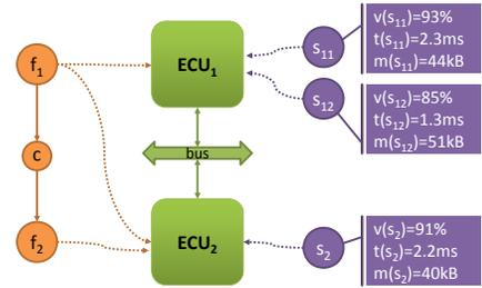
**Figure 2:** Besides the functional task  $t_1$ , which may also be mapped to ECU<sub>2</sub>, two SBST tasks  $s_{11}$  and  $s_{21}$  are available for ECU<sub>1</sub>. Both have different characteristics according to their fault coverage, execution time, and memory footprint. During system design, it has to be decided which SBST task  $s$  to select and schedule it by assigning a period.
