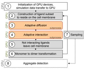
Figure 3: Overview of the model evaluation algorithm with the main simulation loop.
