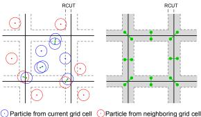
Interaction between particles from neighboring grid cells
