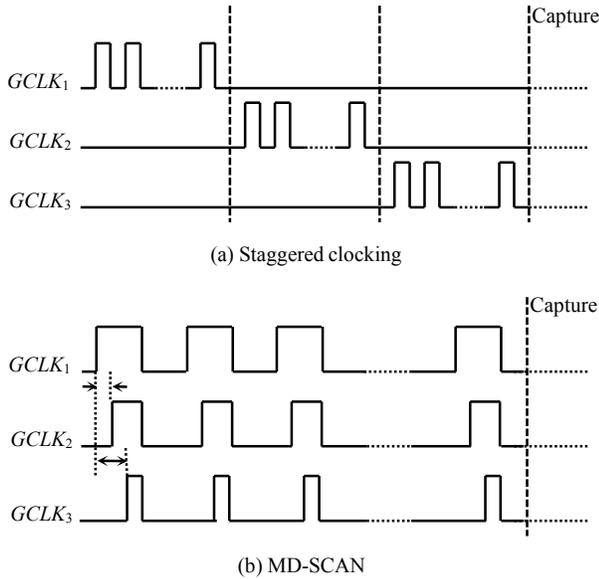
Fig. 5 Clocking schemes for shift power reduction.
