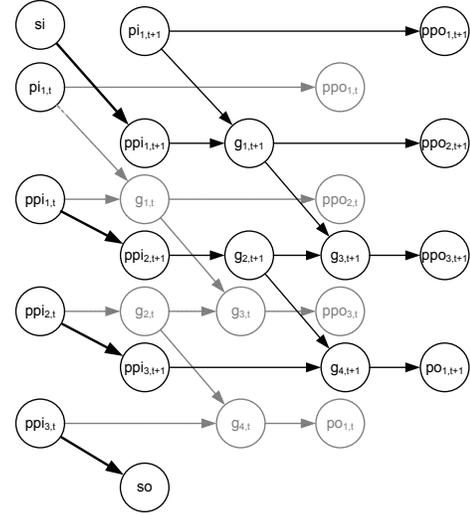
Fig. 4. The graph concatenation for a shift clock.
