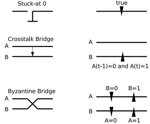
Fig. 7. Examples of conditional stuck-at lines.
