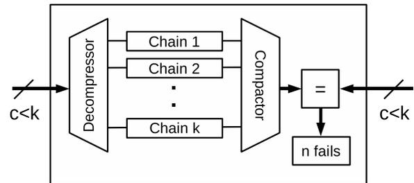
Fig. 2. Test data decompression and response compaction.
