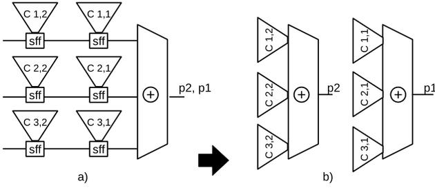
Fig. 6. Combinational representation for extreme response compaction.
