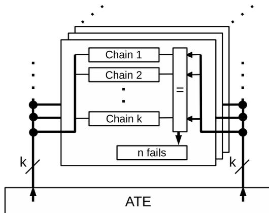
Fig. 1. Principle of multi-site testing.
