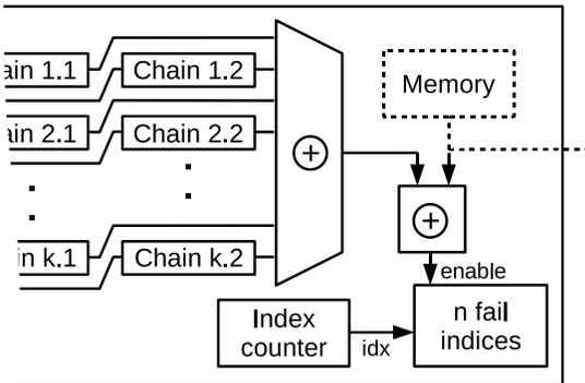
Fig. 5. Target scheme for extreme response compaction.
