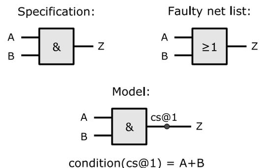
Figure 1: Example of a conditional stuck-at fault
