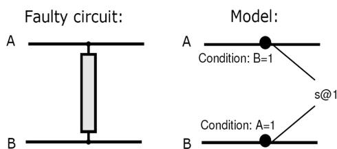
Figure 2: Example of a conditional stuck-at fault modeling a resistive bridge
