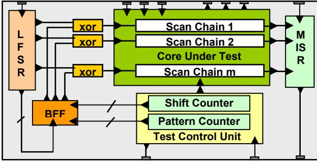
Figure 1: Bit-flipping DLBIST architecture.
