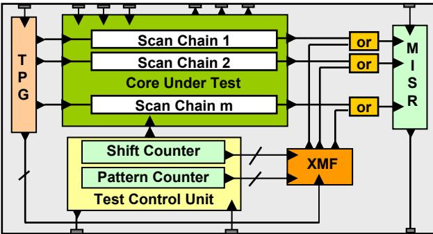
Figure 2: Embedded test architecture with MISR.
