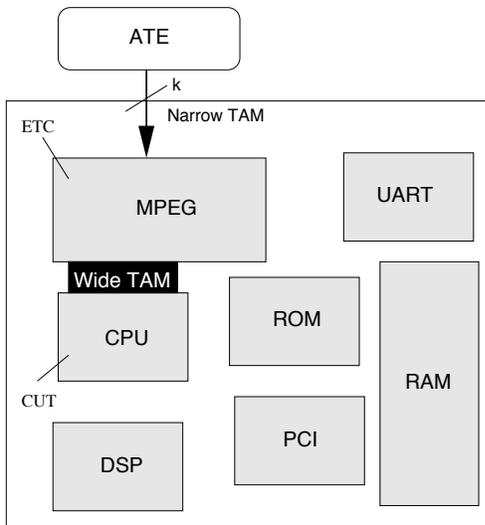
**Figure 1. SoC with the RESPIN Test Architecture**
