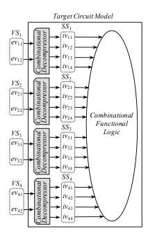
Fig. 8 Decompression Expansion for Scan Slices.
