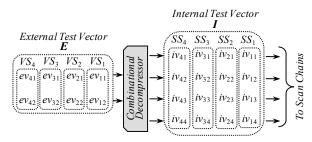
Fig. 7 Test Expansion with Decompressor.
