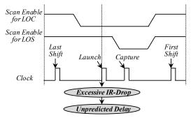
Fig. 1 Waveforms of LOC and LOS Scheme.
