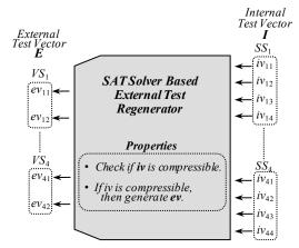
Fig. 10 SAT Solver Based External Test Regenerator.
