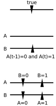
Fig. 7. Examples of conditional stuck-at lines.
