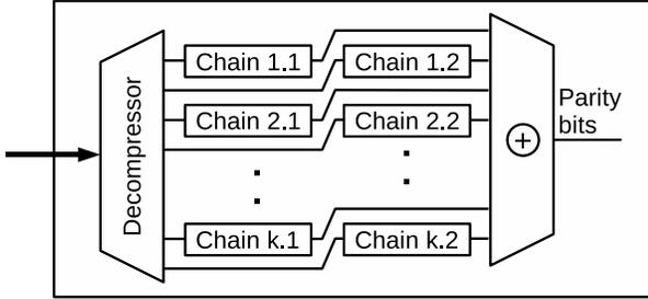
Fig. 4. Extreme response compaction.
