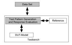
Fig. 1. General test bench
