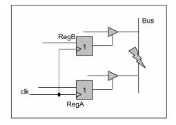
Fig. 6. Assertion check to prevent the hazard
