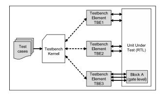
Fig. 3. Adaptive approach for structuring test benches
