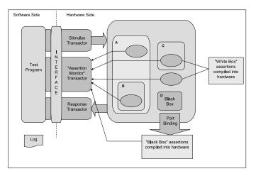
Fig. 4. Transaction level modeling according to [18]
