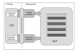
Fig. 5. Principle of embedded test
