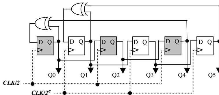
Figure 2: An example of the modified LFSR TPG
