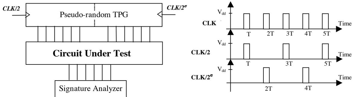
Figure 1: Basic scheme of the low power test pattern generator
