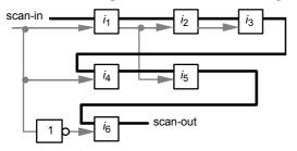
Figure 4: Scan design with regular and compressed shift mode.
