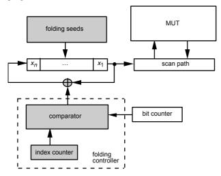
Figure 2: Basic deterministic BIST scheme using a folding
