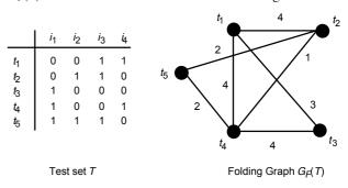
Figure 8: Deterministic test set and folding graph.
