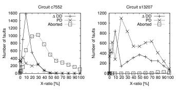
Fig. 4: Increase in definitely detectable faults ( $\Delta$  DD) compared to classical ATPG depending on the X-ratio.
