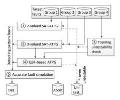
Fig. 3: Overview of the proposed QBF-based ATPG in presence of X-values.
