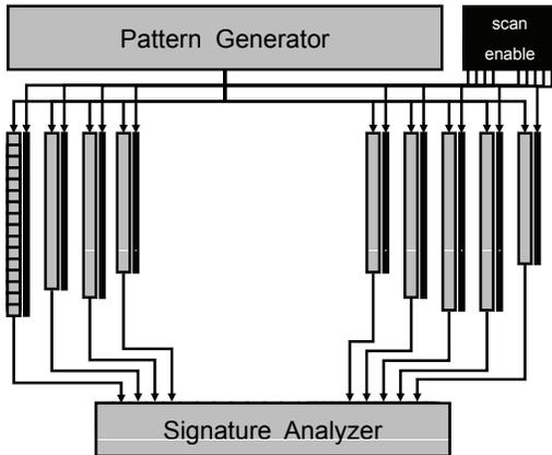
Fig. 1. STUMPS architecture with clock gating
