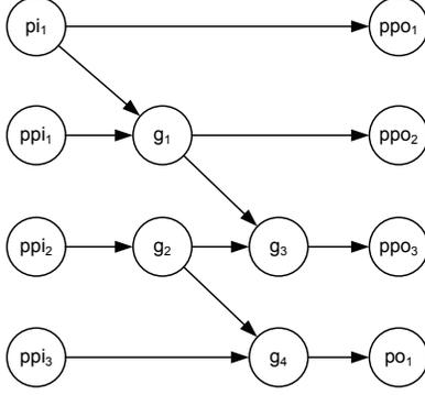
Fig. 2. An example circuit graph. The sets of inputs and outputs to this circuit are  $I = \{pi_1, ppi_1, ppi_2, ppi_3\}$  and  $O = \{ppo_1, ppo_2, ppo_3, po_1\}$ . The edges that represent the (scan) flip-flops and the scan in  $si$  and scan out  $so$  are not depicted here. They are  $FF = \{(ppo_1, ppi_1), (ppo_2, ppi_2), (ppo_3, ppi_3)\}$ . The single scan chain of the circuit is  $sc_1 = (ppi_1, ppi_2, ppi_3)$ .
