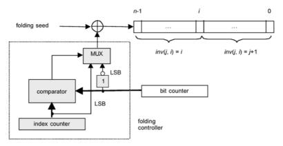
Fig. 12. Structure of the proposed folding controller.
