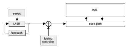
Fig. 5. Target BIST architecture for two-dimensional test data compression.
