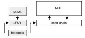
Fig. 2. Test width compression based on the reseeding of LFSRs.
