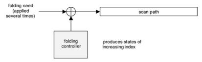
Fig. 11. Alternative approach to generate scan patterns as folding counter sequences.
