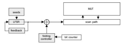
Fig. 13. Complete BIST scheme for two-dimensional reseeding.
