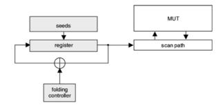
Fig. 3. Vertical test data compression based on the reseeding of folding counters.
