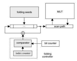
Fig. 10. Basic deterministic BIST scheme using a folding counter.
