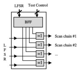
Fig. 3. Sequence-generating logic.
