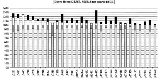
Fig. 6. Silicon area (10,000 patterns, 100% fault efficiency).
