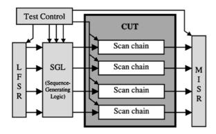
Fig. 2. Target structure of deterministic BIST scheme.
