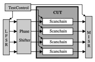
Fig. 1. STUMPS architecture with phase shifting logic.
