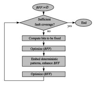
Fig. 4. BFF synthesis algorithm.
