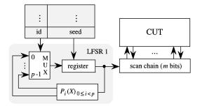
*Fig. 9.* Deterministic BIST scheme based on a multiplepolynomial LFSR by [14].
