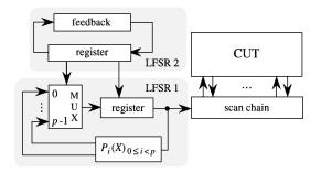
Fig. 7. Multiple-polynomial, multiple-seed LFSR.
