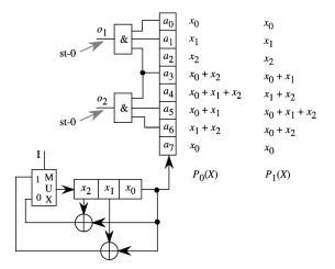
Fig. 3. Scan-based BIST with multiple-polynomial LFSR.
