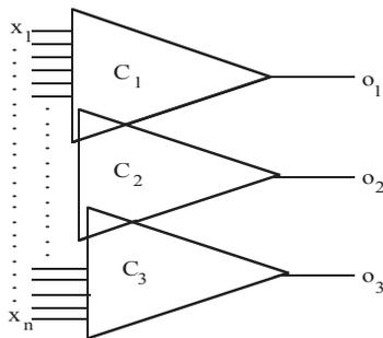
Fig. 1: Pseudo-exhaustively testable circuit with its cones
