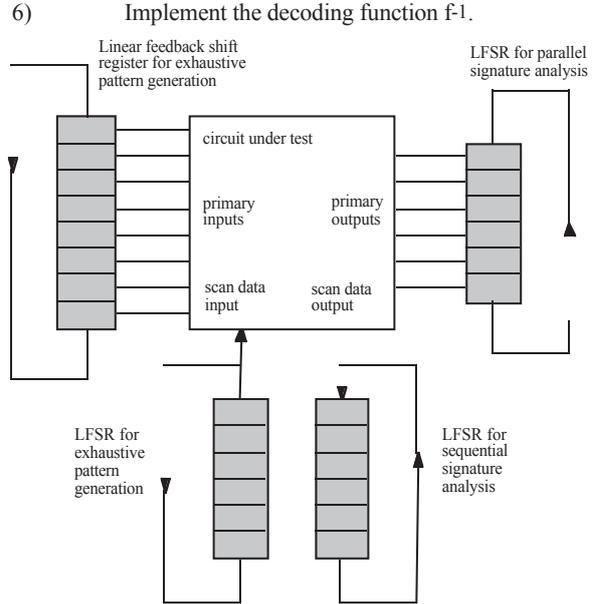
Fig. 10: Pseudo-exhaustive test by an external chip
