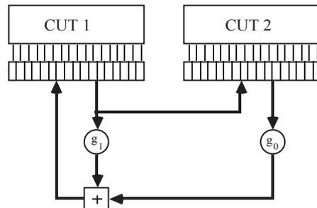
Fig. 7: LFSR of length 2 over  $GF(q)$
