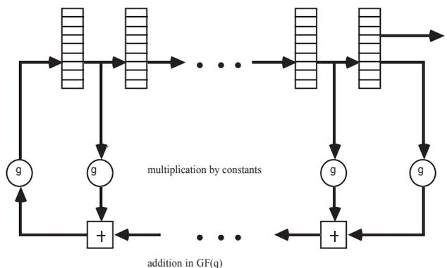
Fig. 6: An LFSR over  $GF(q)$
