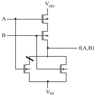
Fig. 2: CMOS-NOR with stuck-open fault
