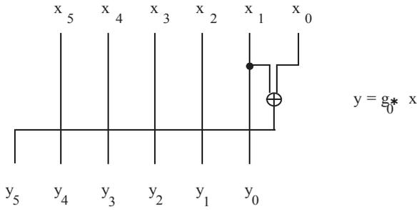
Fig. 8: Implementation of the multiplication  $y = g_0 * x$
