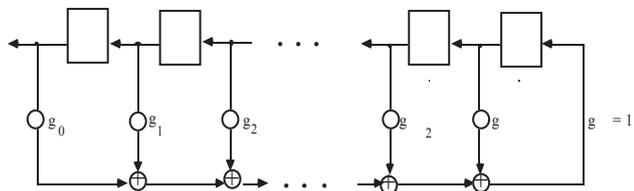
Fig. 5: Standard LFSR over  $GF(2)$
