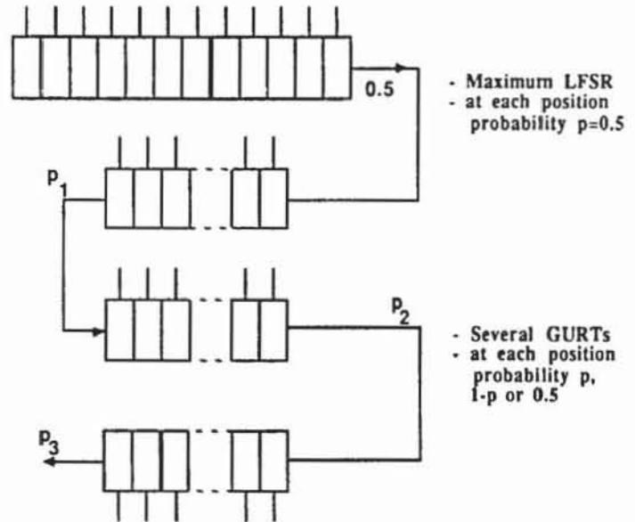
Fig. 10: Self test configuration using GURT's
