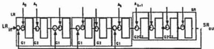
Fig. 9: A GURT in signature register mode
