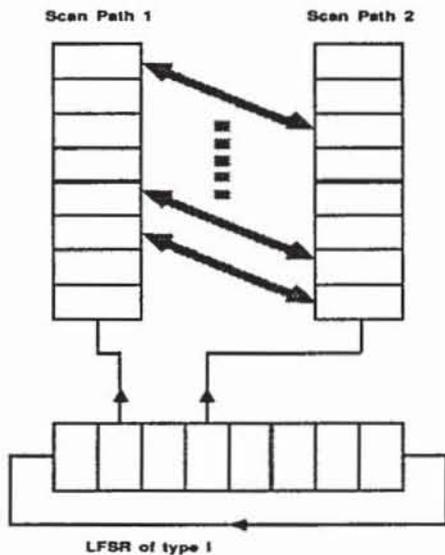
Fig. 3: Autocorrelation by using LFSRs of type I
